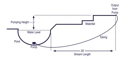
Refer to the chart to determine GPH pump required. Use the calculated pumping height (including adjustments for stream length) to follow down the corresponding lift column until you find the GPH required for the width of the waterfall or stream. Then move over to the left on the chart to the pump size column. This will give the proper GPH pump for your pond.
